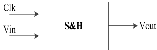
Fig.2: Block diagram of Sample and Hold circuit
